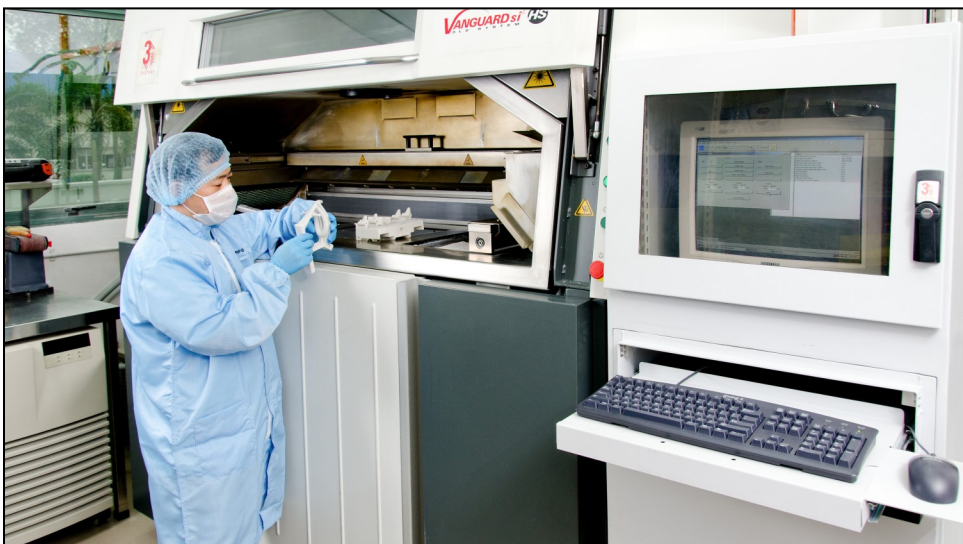
Additive manufacturing, also referred to as SLS rapid prototyping or 3D printing has played an important role in the first phase of swab manufacturing.
